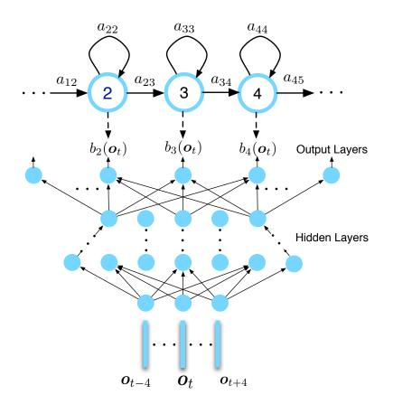
Figure 2.3 DNN-HMM hybrid architectures.
