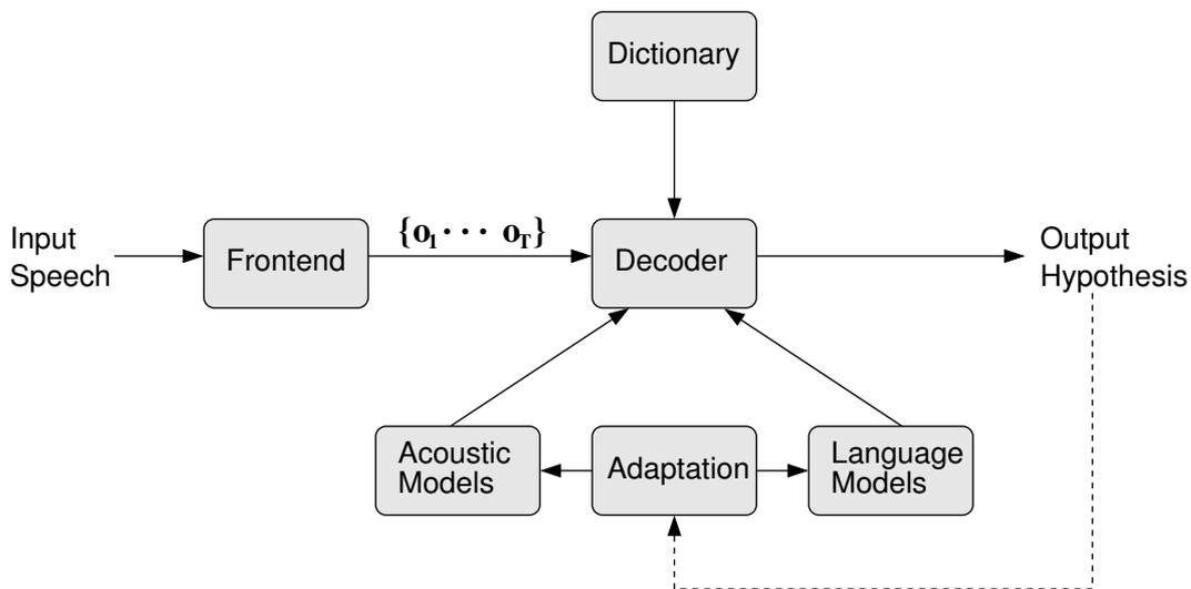
Figure 2.1: *Speech Recognition System Architecture*
