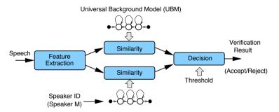
The above diagram shows a standard speaker-verification system.
