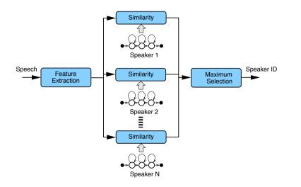
A simple system for speaker identification is given above.
