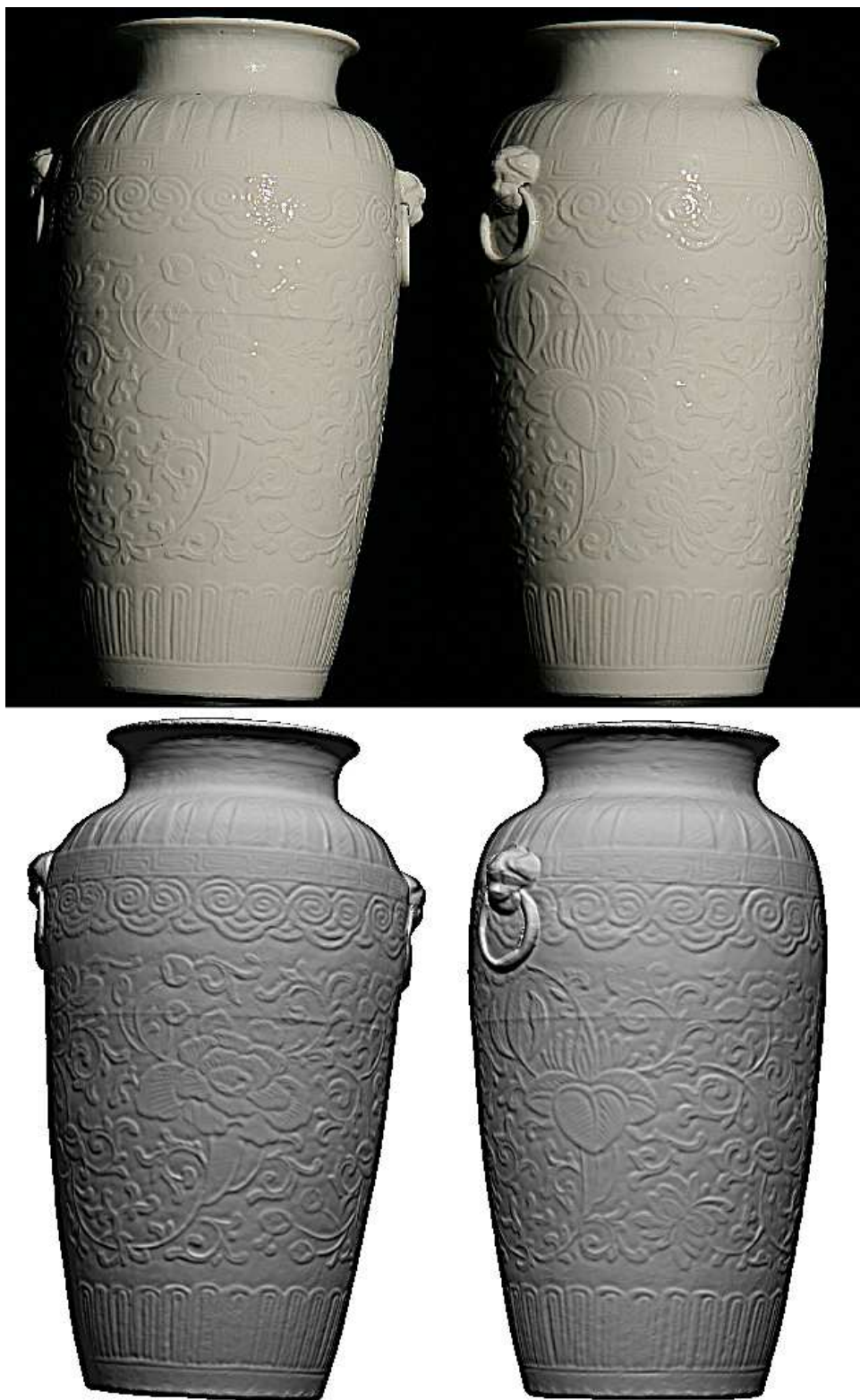
Figure 7.9: Reconstructing porcelain vases. A vase with sub-millimetre relief is reconstructed from a sequence of 36 images. Same setup as Figure 7.8.
