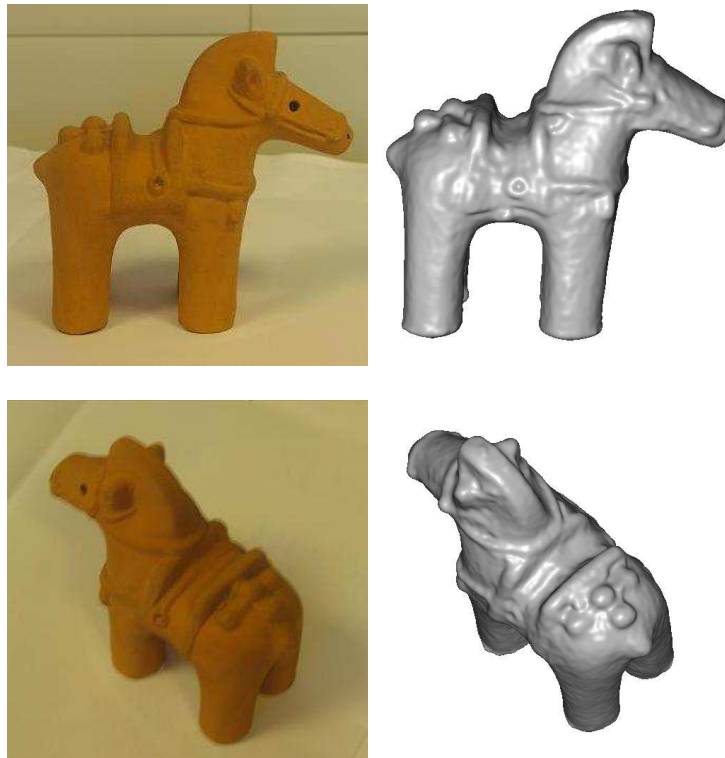
Figure 5.9: Clay horse (real scene). Left column: Images of the clay horse sequence. Right column: Similar viewpoints of the reconstructed model using our method.
