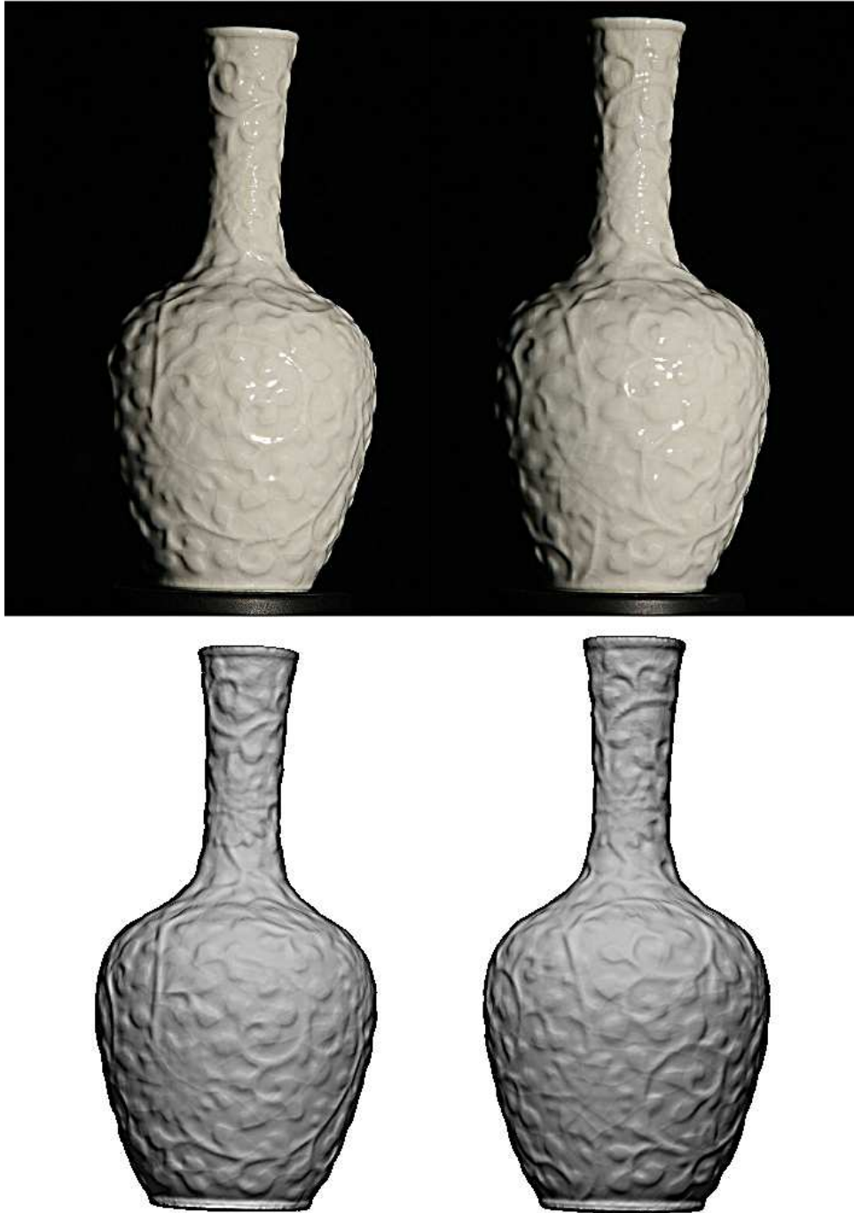
Figure 7.8: Reconstructing porcelain vases. A very fine relief porcelain vase is reconstructed from a sequence of 36 images (two of which are shown in (a)). (b) shows the reconstructed model obtained by our algorithm.
