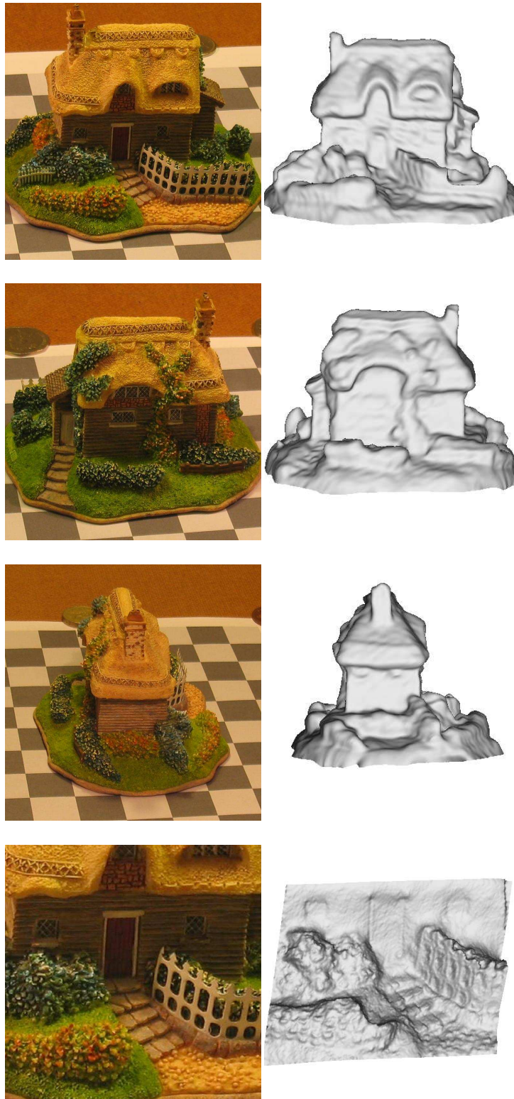
Figure 5.7: House (real scene) . Left column: Images of the toy house sequence. Right column: Similar viewpoints of the reconstructed model using our method.
