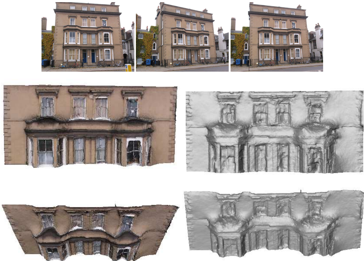
Figure 4.4: Building facade. Top: the images used. Bottom two rows, left and right: texture mapped and untextured relief surface. The base surface was the wall plane. The challenge of the scene is the shiny or transparent windows as well as the fine relief at places. The smoothing of the top side of the balconies is due to the fact that none of our three images information on that part of the scene, as the photographs were taken from street level.
