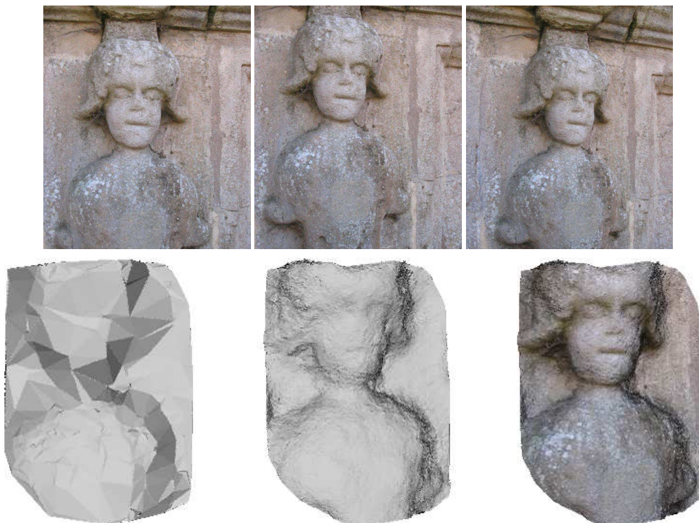
Figure 4.5: Stone carving. Top: the images used. Bottom left: the base surface. Bottom middle: the untextured relief surface. Bottom right: the texture mapped relief surface.
