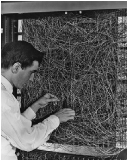
Figure 2: The Mark 1 perceptron
