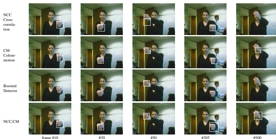
Figure 7: Comparison of individual trackers with combined NCC/CM tracker. This figure shows snapshots of a sequence and results of the NCC tracker, the CM tracker, frame-by-frame detection and the proposed NCC/CM tracker.
