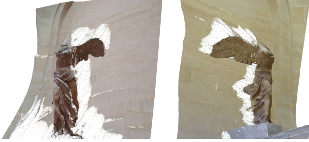
Figure 4. Two single view depth point clouds. The depth interpolation does not create accurate background depth values, as there are not enough samples. But it does create a depth-discontinuity boundary that aligns well with images and recovers geometry where PMVS points are dense.
