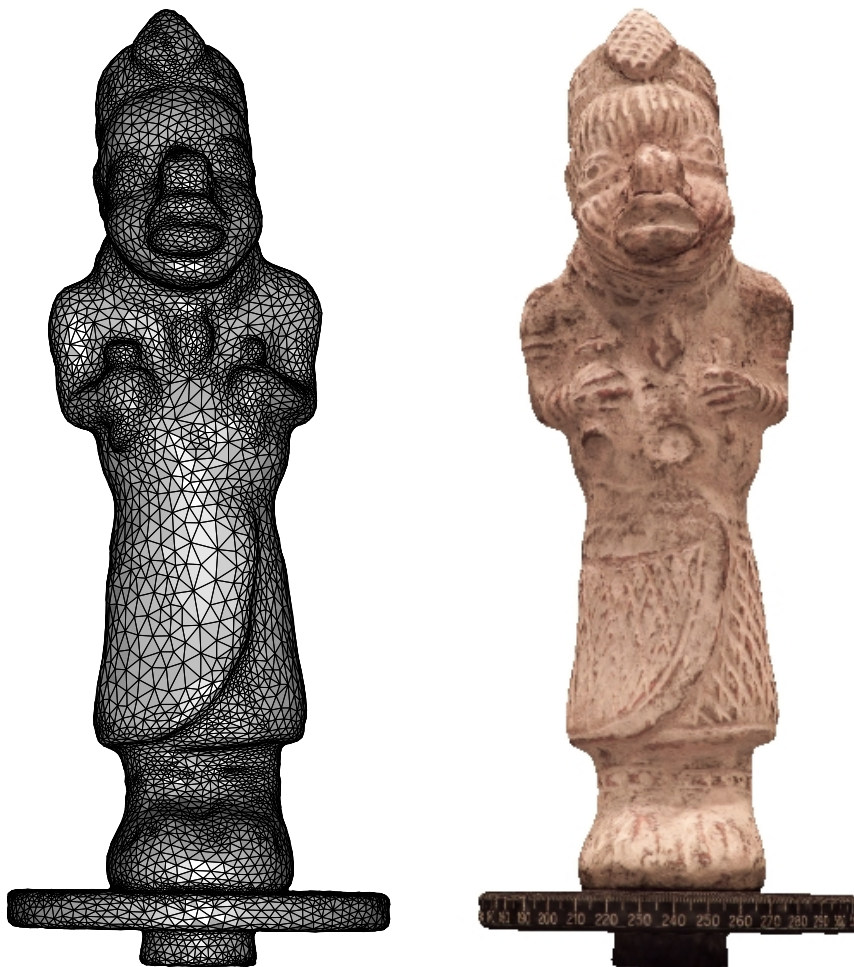
Figure 2.35: Triangle mesh and textured mesh using the texture map of Fig. 2.33. We thank Houman Borouchaki for this simplified version of the bigHead model.
