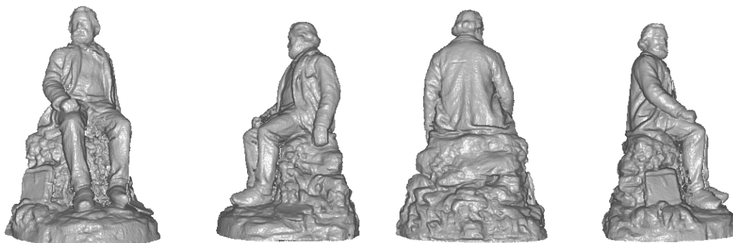
Figure 3.37: Four rendered views of the correlation voting volume for the Millet sequence. The volume has been binarized with an accumulated correlation threshold of 30.
