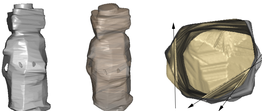
Figure 3.26: Different views of the Guardians visual hull. From left to right: frontal view, transparent view (we can see the tunnels created by the silhouette holes), and top view of an horizontal cut of the visual hull to better see the tunnels shape.
