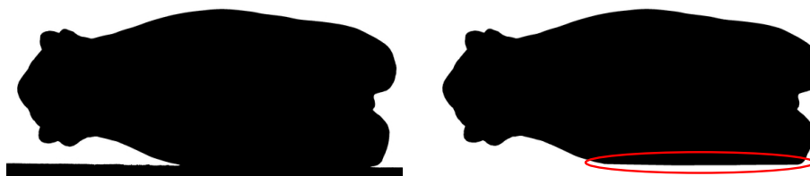
Figure 3.50: Separation of the turntable silhouette from the object silhouette by line clipping. Left: original extracted silhouette. Right: clipped silhouette (the clipped region is shown by the red ellipse).
