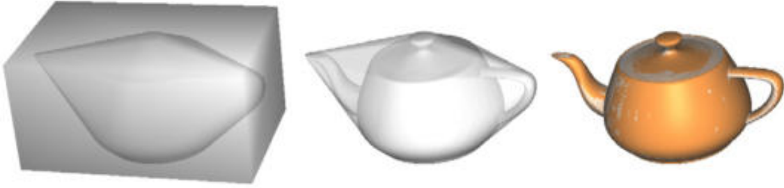
Figure 2.2: Different object initializations. From left to right: bounding box+convex hull, convex hull+visual hull, visual hull + real object.
