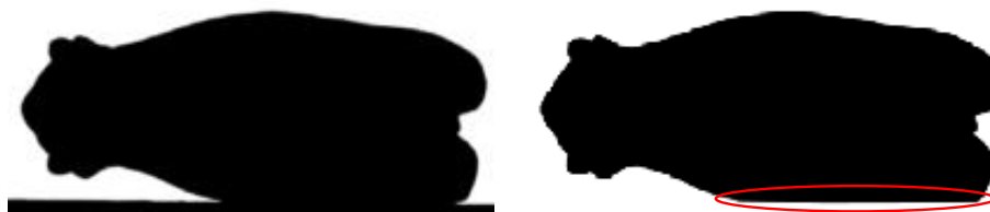
Figure 3.50: Separation of the turntable silhouette from the object silhouette by line clipping. Left: original extracted silhouette. Right: clipped silhouette (the clipped region is shown by the red ellipse).
