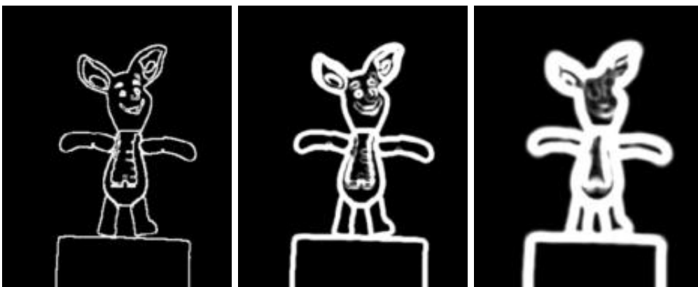
Figure A.5: From left to right three J -images computed over the 5-class quantized image with a window size of 9, 17 and 33 pixels respectively.
