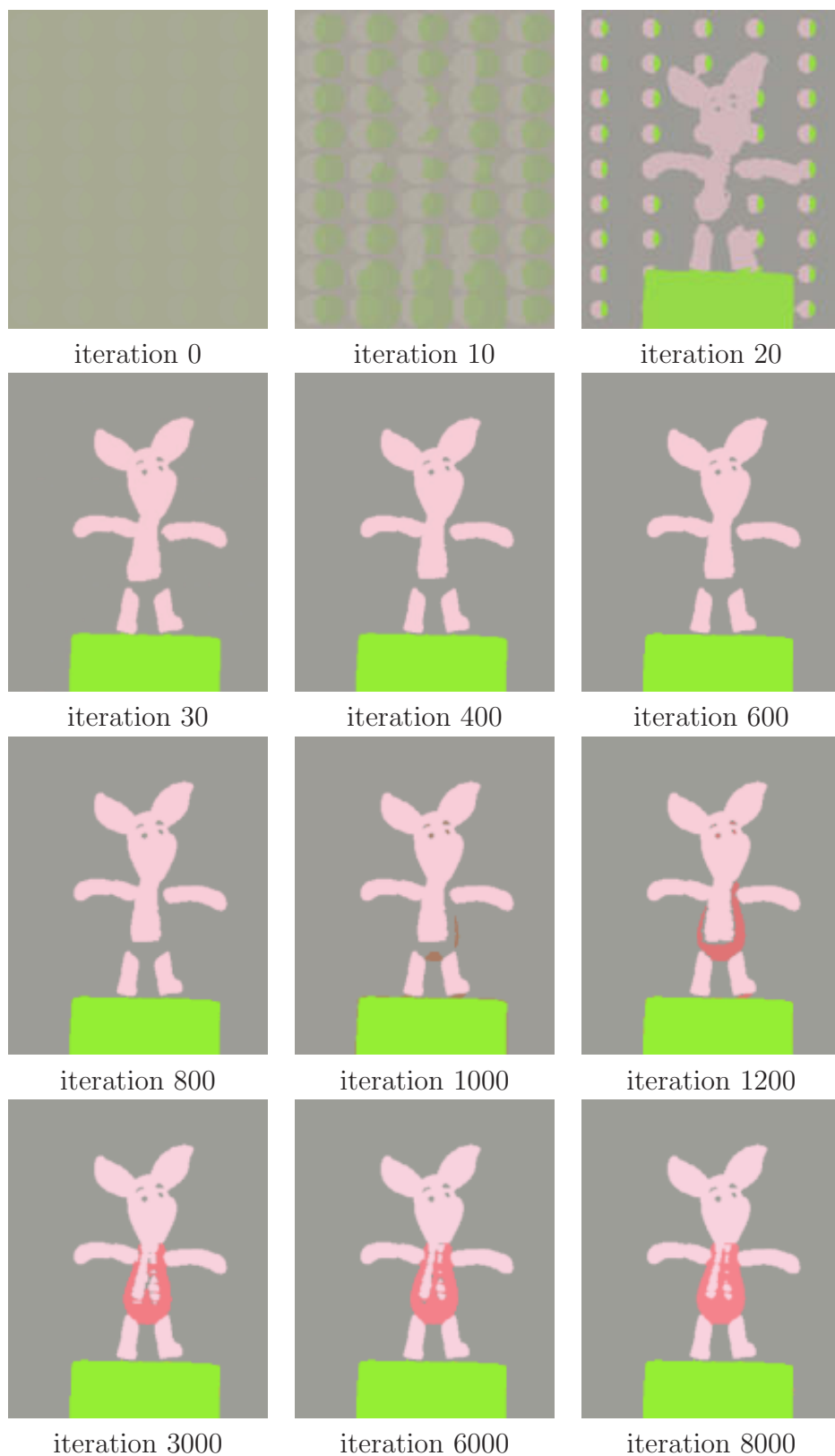
Figure A.15: 4-phase segmentation using the proposed speed. The level sets are able to converge to the global minimum. The four regions are drawn with their corresponding mean color.
