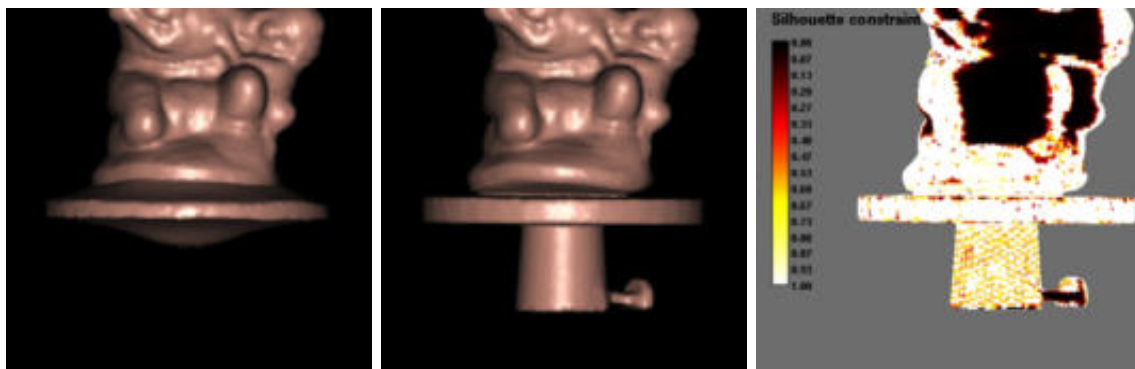
Figure 3.11: Twins model detail after convergence. Left: evolution under texture force only. Parts of the object with no texture disappear. Middle: evolution under both the texture force and the silhouette force. The parts of the object with no texture follow the silhouette force (visual hull). Right: \alpha component of the silhouette force after convergence.
