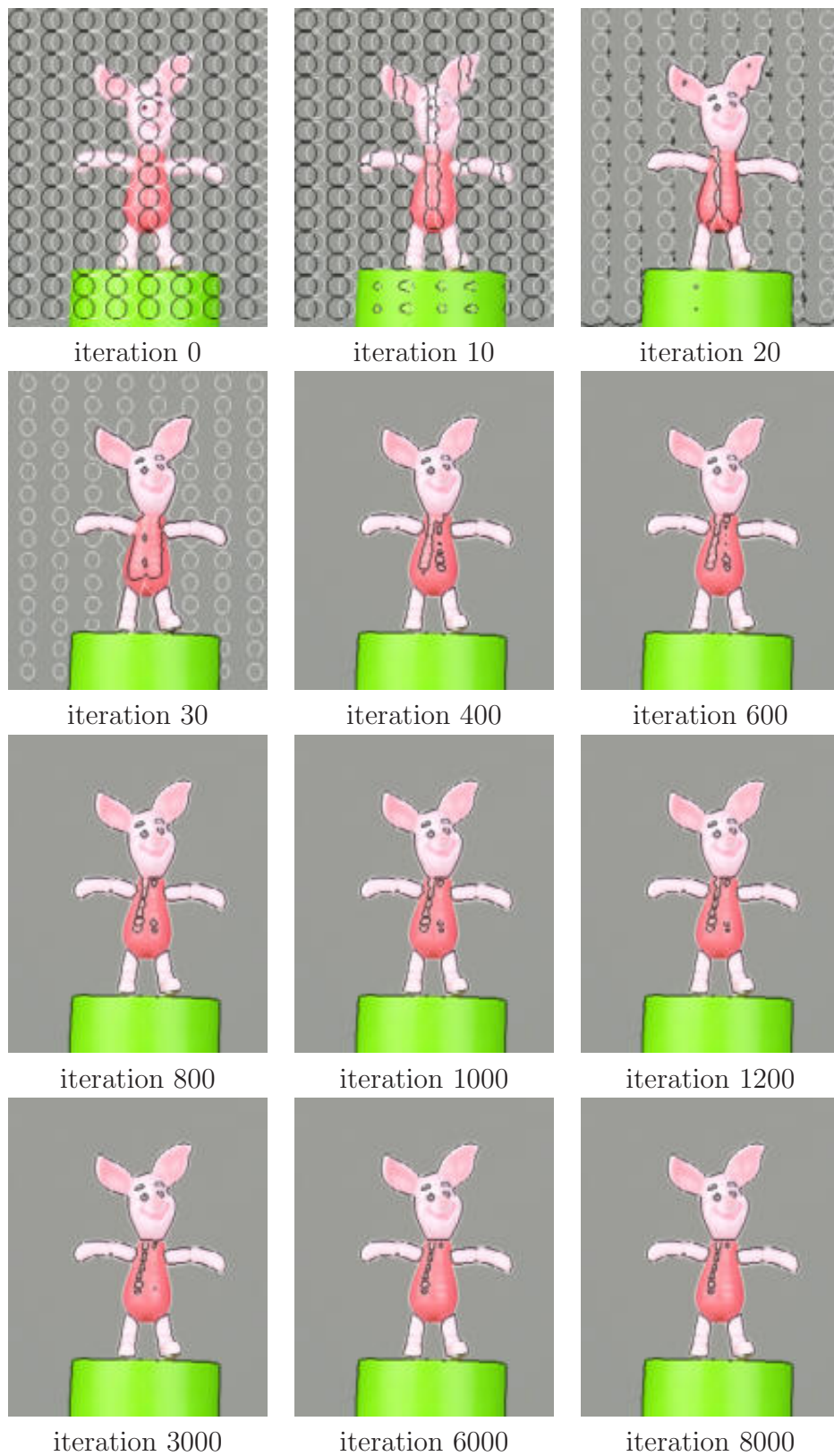
Figure A.10: 4-phase segmentation using [Vese and Chan, 2002] speed. The level sets are able to converge to the global minimum. \phi_0 and \phi_1 zero level set are drawn in black and white color, respectively.
