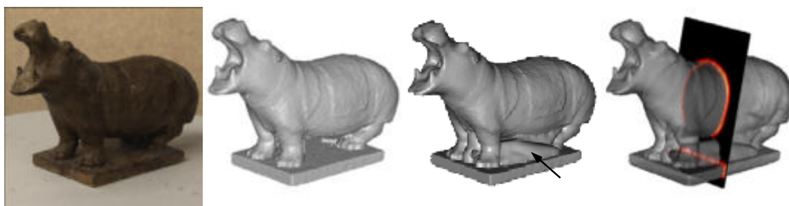
Figure 3.32: Hippopotamus object. From left to right: one of the original images, correlation volume, model after convergence, and superposition of the deformable mesh with the GVF computed for 10 levels.
