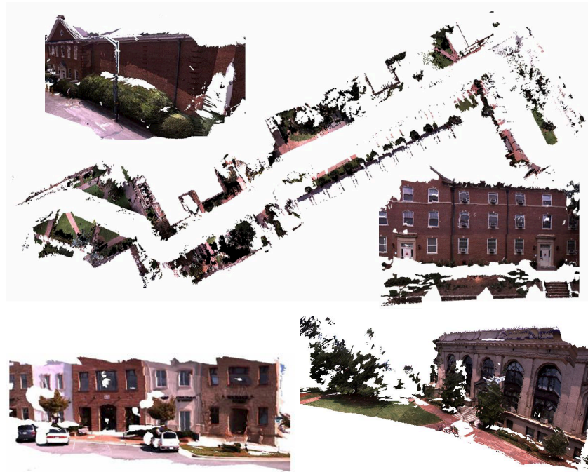
Figure 3.11: Streetside reconstructions by plane sweeping stereo algorithm by Gallup, Frahm, Mordohai, Yang, and Pollefeys [76].
