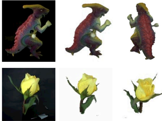
Figure 2.8: Voxel coloring [166] results of Dinosaur toy and Rose. The objects were rotated 360^\circ below a camera. Left shows one of the 21 input images. Right shows two different views of the reconstruction.
