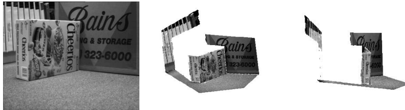
Figure 4.2: Birchfield and Tomasi proposed a piecewise affine disparity estimation algorithm back in the 90s. The left is one of the input images, while the middle and the right show the reconstructed 3D model rendered from two different viewpoints. (Figure courtesy of Birchfield et al.)
