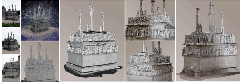
Figure 3.36: Processing pipeline of an MVS system proposed by Vu, Labatut, Keriven, and Pons [193]. After reconstructing a sparse point cloud from images (top second column), a volumetric graph cuts with Delaunay tetrahedralization is used to initialize a mesh model (bottom second column), which is polished by the MVS refinement algorithm (third column). The right hand side of the figure shows the final 3D model with a mix of shaded and texture mapped rendering.
