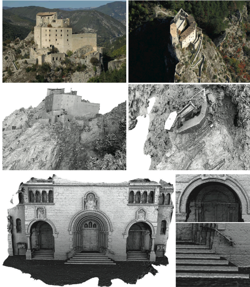
Figure 3.37: Top: A reconstruction result by an MVS system by Vu, Labatut, Keriven, and Pons [193]. A helicopter was used to acquire 109 images (3.1 Mpixels). For each column, the top row shows the reconstructed mesh model and the bottom row shows an input image with a similar viewing angle. Bottom: Another reconstruction result by an MVS system by Vu, Labatut, con Keriven and Pons [193]. 25 images of high resolution images ( 2048 \times 3072 pixels) are the input to the system. The dataset ( Herz-Jesu-P25 ) is from a MVS benchmark project by Christoph Strecha [176].
