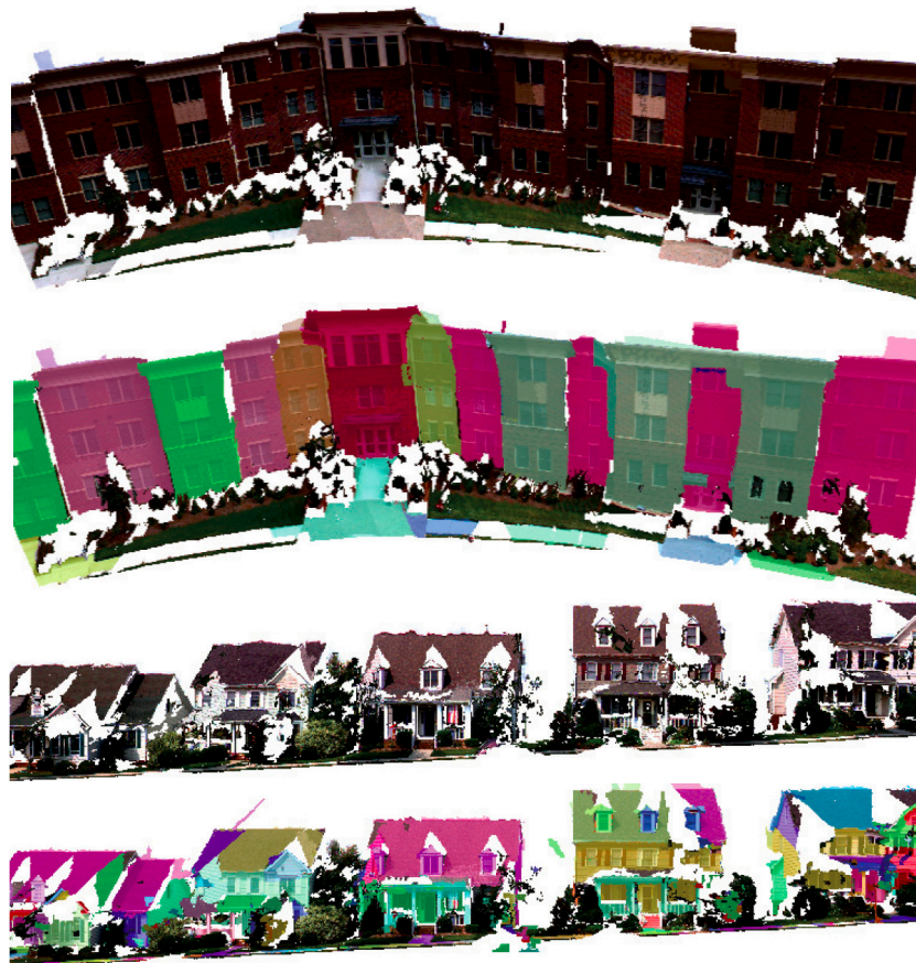
Figure 4.13: Reconstruction results of a depthmap estimation algorithm by Gallup, Frahm, and Pollefeys [77] for two scenes. For each scene, the top shows the final texture mapped depthmaps, and the bottom highlights the estimated plane IDs. (Figure courtesy of Gallup et al.)
