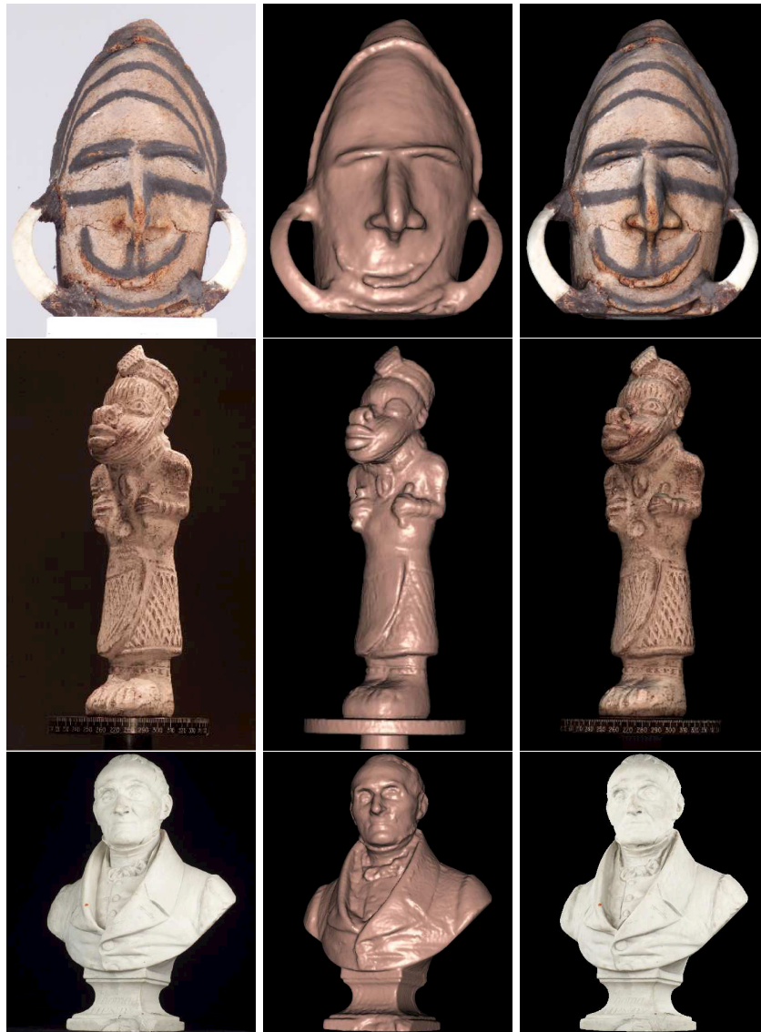
Figure 3.35: Reconstruction results by Hernández and Schmitt [93]. From left to right, one of the 36 input images, the reconstructed mesh model, and the texture mapped mesh model for each dataset. The visual hull model is used to initialize the mesh, which is then iteratively refined.
