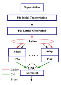
Fig. 1. BN-M multi-pass and multi-branch evaluation framework
