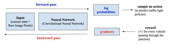
Figure 2. Policy Gradient Reinforcement Learning Pipeline
