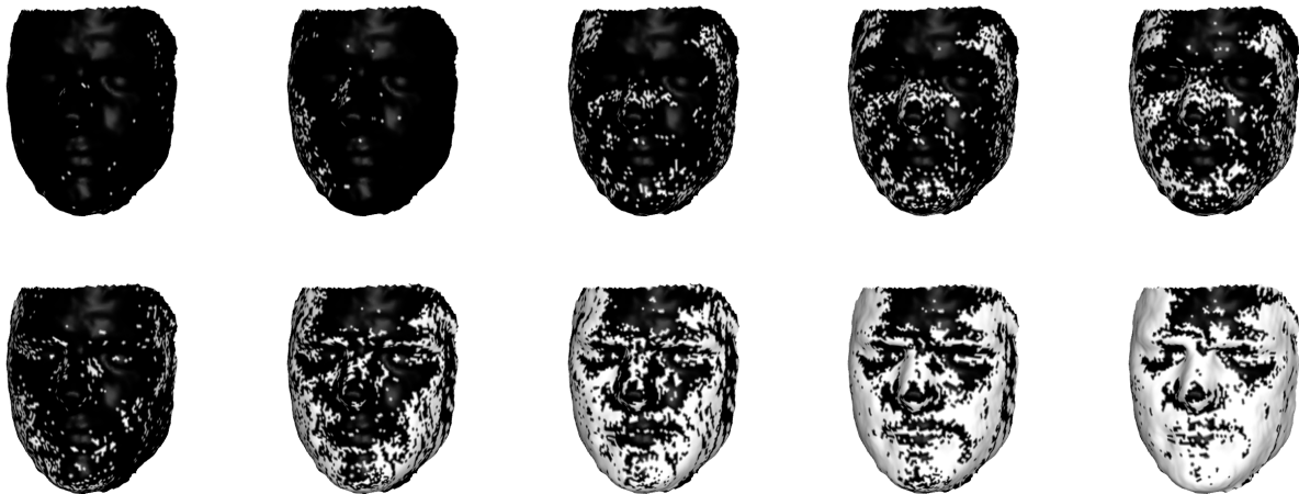
Fig. 7 Distribution of inliers (in white) as a function of the threshold \tau . From left to right, \tau = 1 , \tau = 2 , \tau = 3 , \tau = 4 , \tau = 5 . The image intensities are quantized in the range from 0 to 255. The first row shows the inliers for the 3pt algorithm while the second row is the same for the 4pt algorithm. This experiment used the calibration sequence of figure 3
