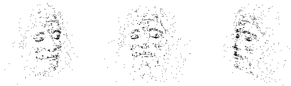
Fig. 14 Sparse set of 3d points after using a structure-from-motion algorithm on the sequence of Fig. 9. From left to right, the 3d points are shown from three different viewpoints roughly at -45 degrees, 0 degrees, and 45 degrees.
