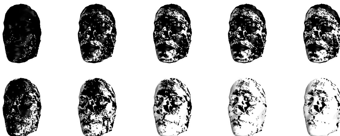
Fig. 17 Distribution of inliers (in white) as a function of the threshold \tau . From left to right, \tau = 1 , \tau = 2 , \tau = 3 , \tau = 4 , \tau = 5 . The image intensities are quantized in the range from 0 to 255. The first row shows the inliers for the 3pt algorithm while the second row is the same for the 4pt algorithm. This experiment used the calibration sequence of figure 9
