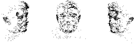
Fig. 4 Sparse set of 3d points after using a structure-from-motion algorithm on the sequence of Fig. 3. From left to right, the 3d points are shown from three different viewpoints roughly at -45 degrees, 0 degrees, and 45 degrees.
