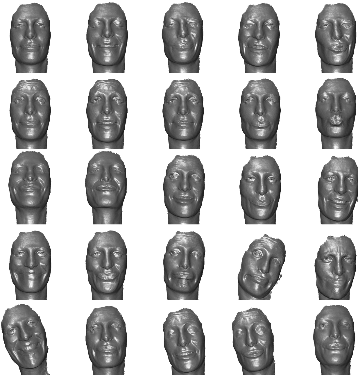
Fig. 18 Acquisition of 3d facial expressions using [11]. The system was calibrated using the self-calibration technique described in this paper.
