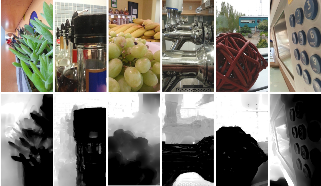
Figure 5. Multiple datasets captured with a hand-held Samsung Galaxy phone. From left to right (number of frames in parenthesis): plants(23), bottles(31), fruits(30), metals(33), window(27), telephone(33). Top row shows the all-in-focus stitch. Bottom row shows the reconstructed depth maps.
